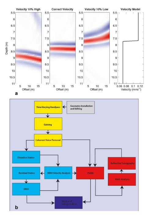
**Fig. 1.** (a) Sensitivity of PSDM to velocity errors illustrated with a simple two-layer model; and (b) processing flow for reflection tomography in the PSDM domain. The flow on the upper left is a standard CMP processing flow with the primary objective of producing a starting velocity model for PSDM. The PSDM flow can be iterated if necessary to minimize RMO.
