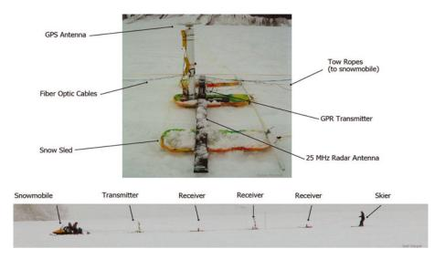
**Fig. 4.** Photograph of the multichannel georadar system used for multi-offset data acquisition. In this first-pass configuration, the source/receiver offsets were 5, 10 and 15 m. Four additional passes were completed with variable offsets to complete a dataset with offset ranging from 5 to 150 m.
