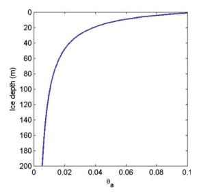
Fig. 2. Vertical distribution of air volume vs ice depth computed assuming ideal gas behavior and hydrostatic pressure.
