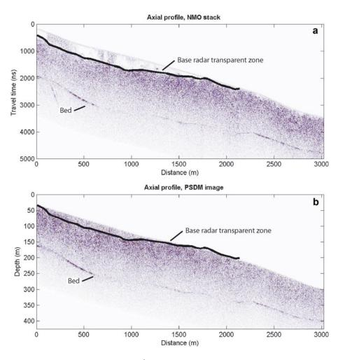
**Fig. 5.** (a) CMP stack using a constant velocity of 0.168 m ns<sup>-1</sup> for the NMO correction; and (b) PSDM image. The bed reflection is clearly evident in both images. The radar-transparent zone is most clearly seen in the CMP stack. We used an aggressive stretch mute for the PSDM image, which eliminated the upper part of the section but minimized stretch-related errors in the RMO analysis.
