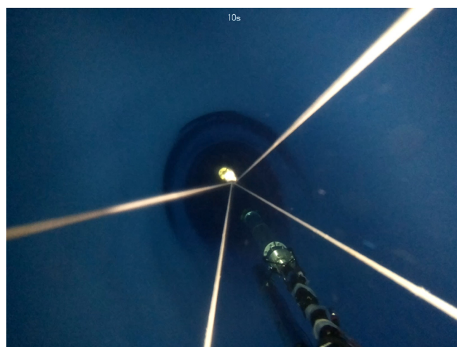
Fig. 10. Hole 3, Deployment 2, CAM1: Image shows the borehole pump located in the cavity linking the three boreholes. Approximately 232–237 m below the surface.
