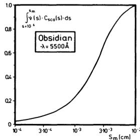
Fig. 3. The normalized integral of the effective scattering cross section over size distribution, as a function of its upper limit  $s_m$
