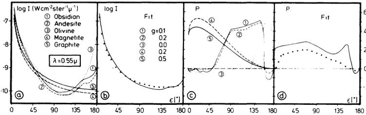
Fig. 1. a,c-calculated ZL brightness and polarization along the Ecliptic for individual materials; b,d-comparison of the results for a mixture with weights  $g$  with observations taken from Leinert's review (1975).
