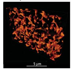
Voltex visualization of porosities in a fuel cell electrode
