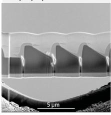
TEM lamella created to measure the amorphous damage created during FIB sample preparation
