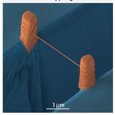
Platinum nanowire deposited and milled to about 50 nm diameter for use as a gas sensor
