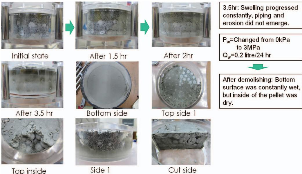
FIG. 12. Case 8; experiment with constant inflow rate which caused piping. Distilled water was fed with inflow rate of 0.001 l/min.
