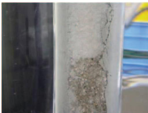
FIG. 23. Water splashed from sediment as jet water flowed making a turbulent flow.
