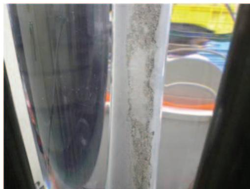
FIG. 22. The formation of sedimentation by silica sand. The light grey part is the sedimentation of no. 5 silica sand.
