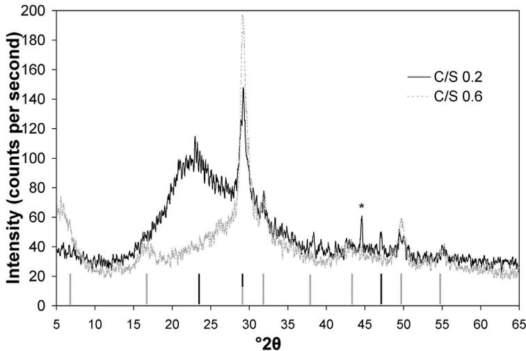
FIG. 4. X-ray diffraction patterns for C-S-H gels with C/S of 0.2 and 0.6; grey vertical lines show the peak positions for C-S-H (I) above 50% relative intensity; black vertical lines are for  $\text{CaCO}_3$ ; \* this peak is probably an artefact of the sample holder.
