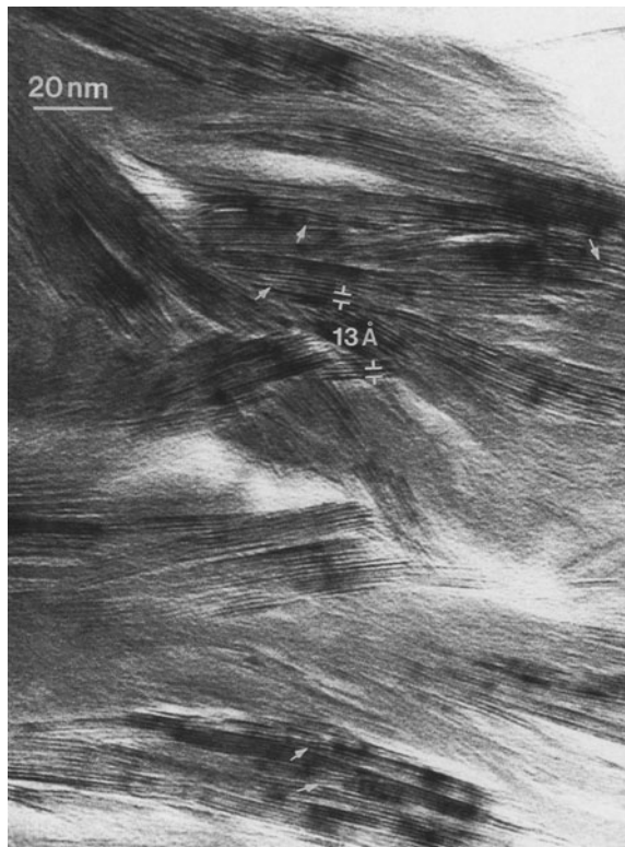
Figure 2. TEM lattice fringe image of permanently expanded bentonite showing that smectite occurs as imperfect and anastomosing layers having a 10.5- to 13-Å interlayer spacing with numerous edge dislocation-like layer terminations (indicated by white arrows).
