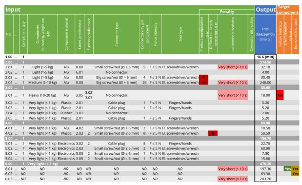
Figure 1. Visualization of the disassembly design tool with its main components; columns marked with "..." are removed for confidentiality reasons and to save space; rows marked with "ND" cannot be displayed for confidentiality reasons
