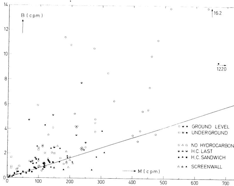
Fig 4. Background counting rate (B) as a function of meson counting rate (M). The underground laboratories (below 7m) are specifically indicated. Further identification was made for Oeschger-type counters and for the counter shielding: no neutron shielding by a layer of a hydrocarbon compound (HC), merely an inner layer of HC and a layer of HC between two layers of high specific density material (HC sandwich). The solid line indicates a favourable trend of B/M of 0.83% (2.5cpm/300cpm).
