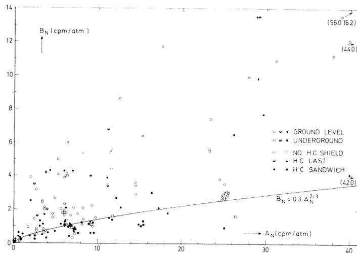
Fig 5. Relation between  $^{14}\text{C}$  counter background,  $B_N$ , normalized to 1 atm (Eq 6) and the effective counter size, represented by the normalized standard activity,  $A_N$  (Eq 1). Identifications are made of the position of the counter with respect to ground level (underground = > 7m below ground level) and type of shielding.
