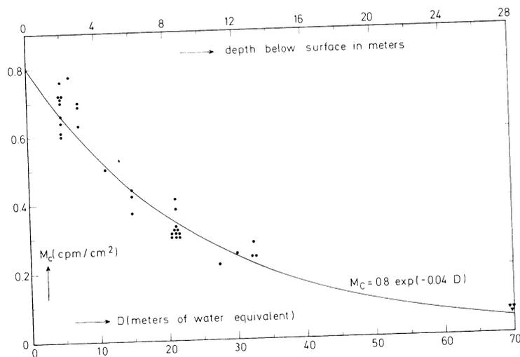
Fig 3. Meson counting rates of a number of  $^{14}\text{C}$  proportional counters per  $\text{cm}^2$  of effective counter cross-section as a function of the shielding. The shielding capacity of sand and concrete was transferred to meters of water equivalent by using an average specific gravity of  $2.5\text{g}/\text{cm}^3$ . The shielding effect observed is  $4\%/m$  of water or ca  $10\%/m$  of depth (Eq 4).
