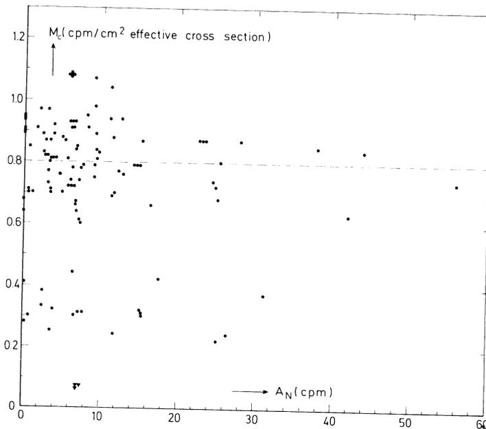
Fig 2. Meson counting rates of  $^{14}\text{C}$  proportional counters per  $\text{cm}^2$  of effective counter cross section (Eq 3) as a function of the effective counter size (normalized standard counting rate (Eq 1)). The triangular points are maximum counting rates.
