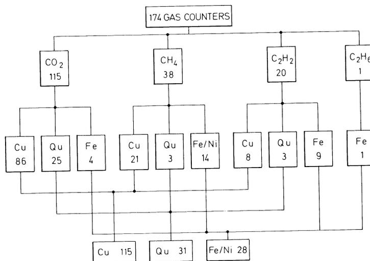
Fig 1. Survey of construction materials and counting gases used for  $^{14}\text{C}$  proportional counters. This compilation represents > 80% of the  $^{14}\text{C}$  counters in operation. Cu = copper, Qu = quartz, Fe = iron, Ni = nickel.
