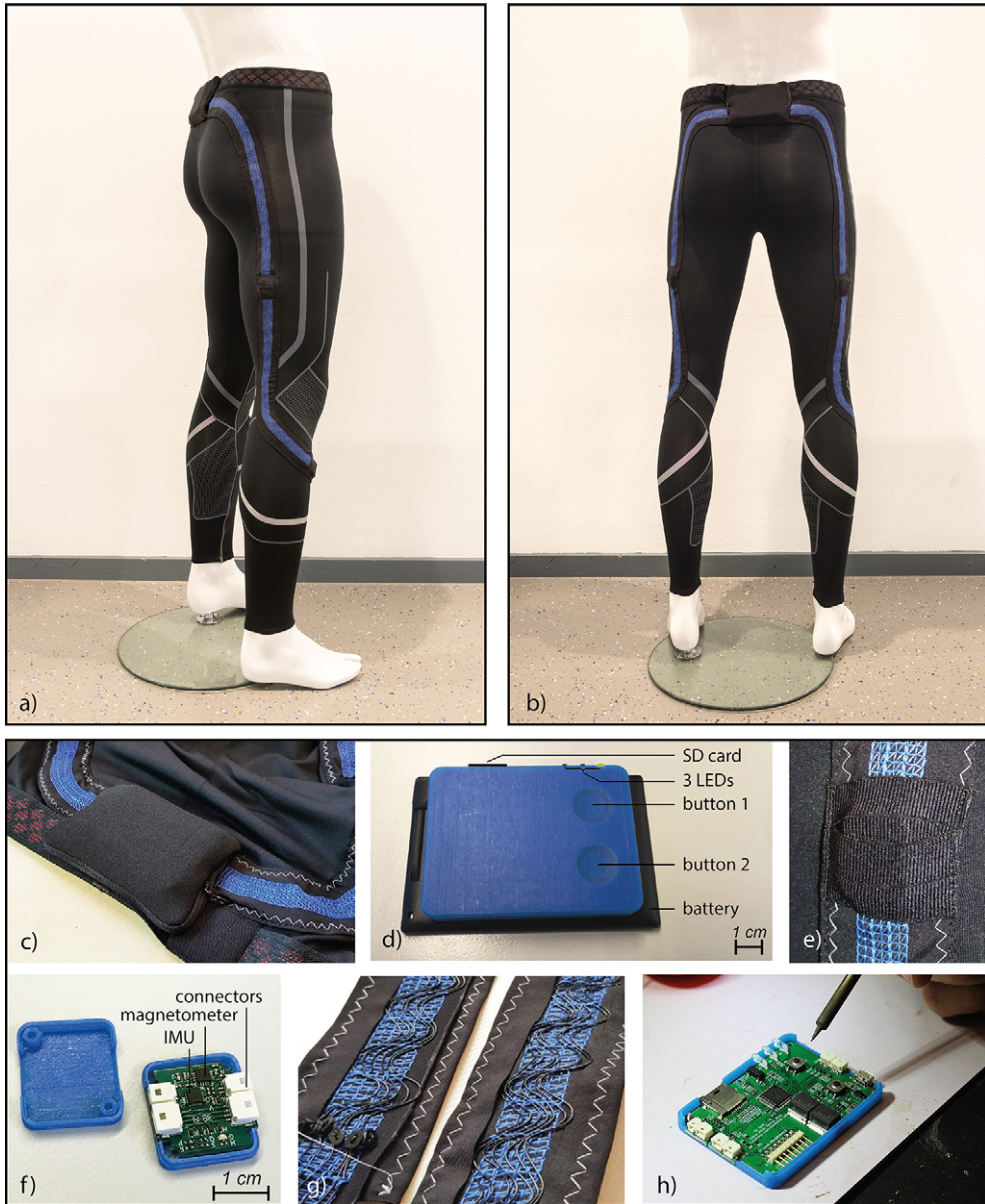
Figure 2. (a) Side view sensor tights, (b) Back view sensor tights, (c) Pocket with central unit PCB and battery, (d) Battery and central unit with user interface, (e) Pocket of a sensor node, (f) A sensor node, (g) Interlaced wiring that allows for 100% stretching, and (h) Central unit during assembling.
