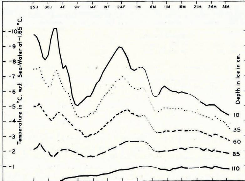
Fig. 4. Ice temperatures at various depths in degrees Centigrade below the sea-water temperature of  $-1.65^{\circ}\text{C}$ . Data from Hudson Bay near Churchill, Manitoba, January to April 1961
