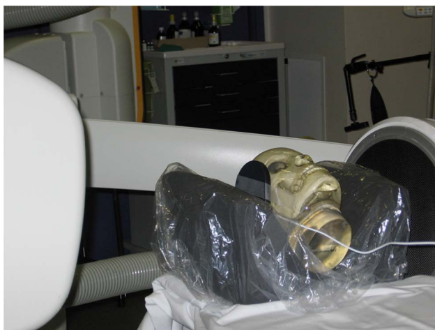
Figure 1: Simulation of 2D DSA with anthropomorphic skull phantom; the 60 cc ion chamber is set up to measure entrance dose during lateral projection cine run.
