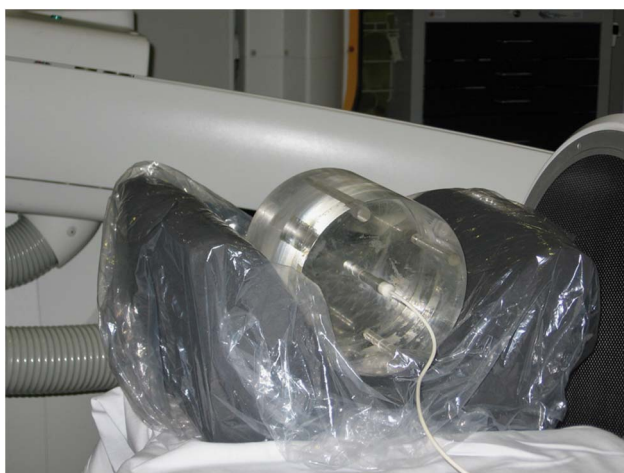
Figure 2: Dosimetry measurements during 3D RA with CT head phantom and a pencil-type 100 mm CT ionization chamber positioned at the center location.
