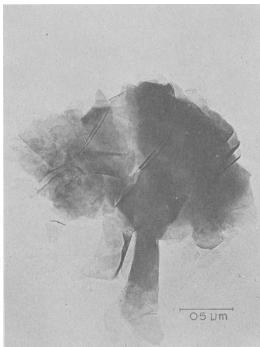
Fig. 4. Coarse fraction of Na-montmorillonite (Wyoming) dispersed onto a Cytochrome C film from a hanging drop.
