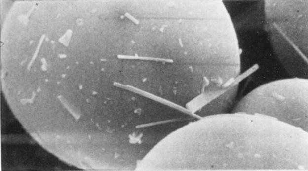
Fig. 3. A  $27\mu$  sphere with surface irregularities that induce a rotational spin (magnification 2600x).
