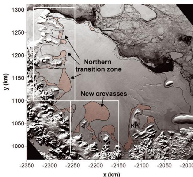
**Fig. 8.** Application of the fracture criterion. Shaded areas indicate regions where modelled stress intensities exceed the fracture toughness of the ice and thus support crevasse opening (image: Moderate Resolution Imaging Spectroradiometer (MODIS) 2002). White boxes outline the images shown in Figure 9. CP: Churchill Peninsula; KP: Kenyon Peninsula.
