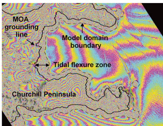
**Fig. 3.** Example section of Larsen C showing a comparison of MOA grounding line (<http://nsidc.org/data/nsidc-0280.html>) and boundary of model domain. Interferogram: ERS-1/2 tandem mission (16/17 November 1995).
