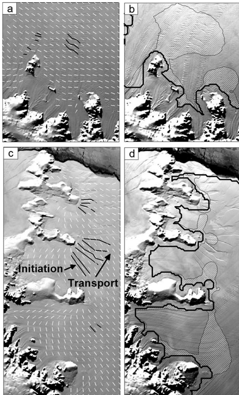
**Fig. 9.** Detail of crevasse orientation and critical stress intensity for selected areas. (a) Crevasse orientation (white) in comparison with observed crevasses (black) downstream of Francis Island. (b) Regions where the critical stress intensity factor of  $50 \text{ kPa m}^{-1/2}$  is exceeded. (c, d) Same parameters for the northern transition zone.
