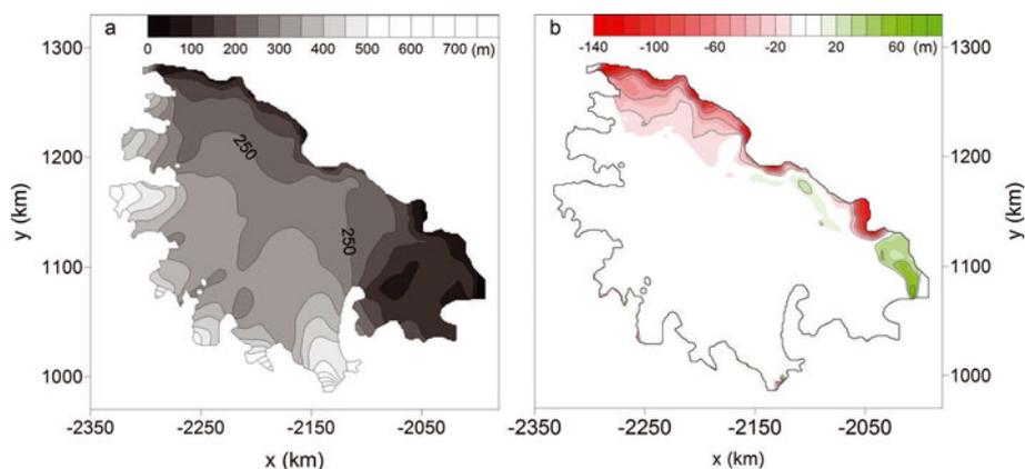
**Fig. 5.** (a) Ice-thickness distribution inferred from integrated BEDMAP (Lythe and others, 2001) radar data and ICESat elevation data (<http://nsidc.org/data/nsidc-0304.html>). (b) Difference from the thickness distribution published in BEDMAP.
