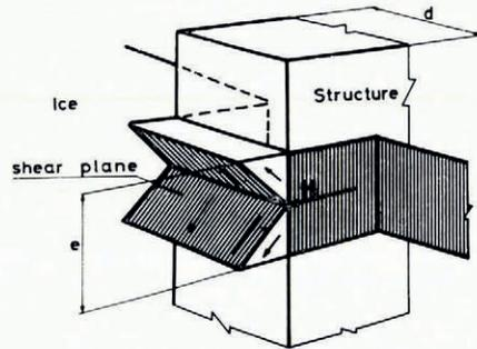
Fig. 1. Shear rupture.
