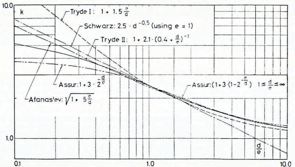
Fig. 2. Indentation strength as a function of  $d/e$ .
