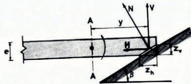
Fig. 4. Forces on inclined plane.
