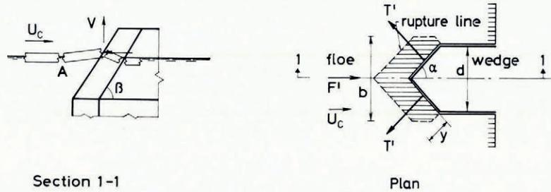
Fig. 6. (a) Vertical section of wedge. (b) Plan of wedge.
