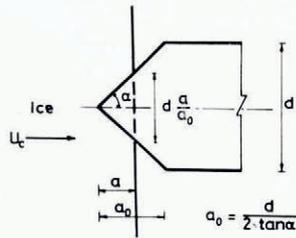
Fig. 3. Partial penetration.
