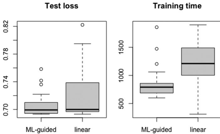
**Figure 4.** Left: loss function value for test dataset in our machine learning-guided partial differential equation (PDE) method (machine learning [ML]-guided) vs. the PDE with spatial additive linear effects model (linear). Right: training computation time (in seconds) for ML-guided vs. linear model.
