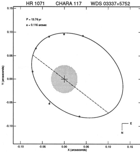
**FIGURE 1.** Seven speckle measurements of HR 1071 are plotted against the newly determined visual orbit of the system. Each point is connected to the orbit by an  $O-C$  line; the broken line is the line of nodes. The hatched circular region represents the  $0''.03$  limit of resolution by speckle interferometry at the 4-m KPNO telescope.
