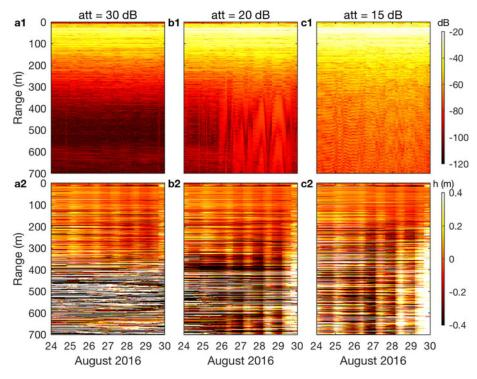
**Fig. 1.** ApRES return signal from site J1Y17. The full deramped chirp, generated by a transmitted chirp in the 200–400 MHz frequency band has been processed for the three attenuation settings: (a) 30 dB, (b) 20 dB and (c) 15 dB. Return amplitude is plotted in the first row and the detrended cumulative vertical displacement, *h*, in the second row.
