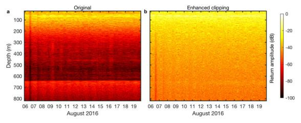
Fig. 5. Return amplitude at Helheim site H3Y16 (a) using the last quarter of the deramped chirp (350–400 MHz band) which avoids clipping, and (b) the full deramped chirp (200–400 MHz band) with clipping sufficiently enhanced to highlight how clipping obscures the bed return signal with artifacts.
