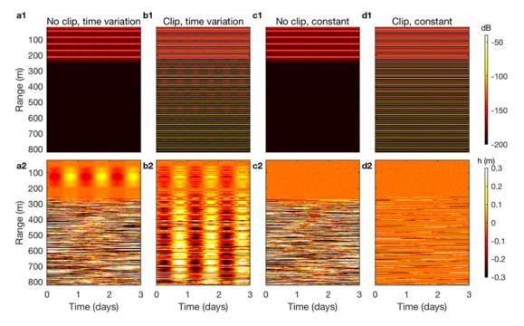
**Fig. 3.** Synthetic deramped signal used to simulate internal reflector motion. The first row shows the return amplitude and the second row the cumulative vertical displacement, *h*. (a) The signal phase varies sinusoidally in time, (b) same as (a) but the signal is clipped, (c) the signal is constant in time and (d) same as (c) but the signal is clipped.
