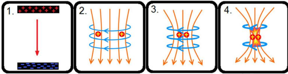
FIGURE 2. Pinch effect in four steps. 1. Current generation by electrodes. 2. The current (presented by orange line) generated by a magnetic field (presented by blue lines). 3. The Lorentz force compresses the plasma. 4. If high enough density and temperature are achieved for a sufficient time, fusion occurs.
