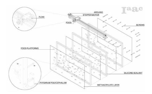
The assembly diagram of the final prototype demonstrates how a food distributor provides Physarum polycephalum with nutrient resources
