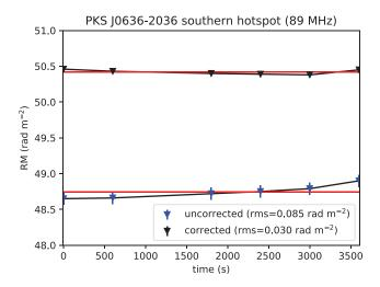
**Figure 10.** Variation in observed rotation measure in the southern hotspot of PKS J0636–2036 as a function of time in the lowest MWA band (89 MHz). Blue points show the measured RM before ionospheric calibration and the Black points show the measured RM after ionospheric calibration. The red line shows the mean value of RM in each instance.
