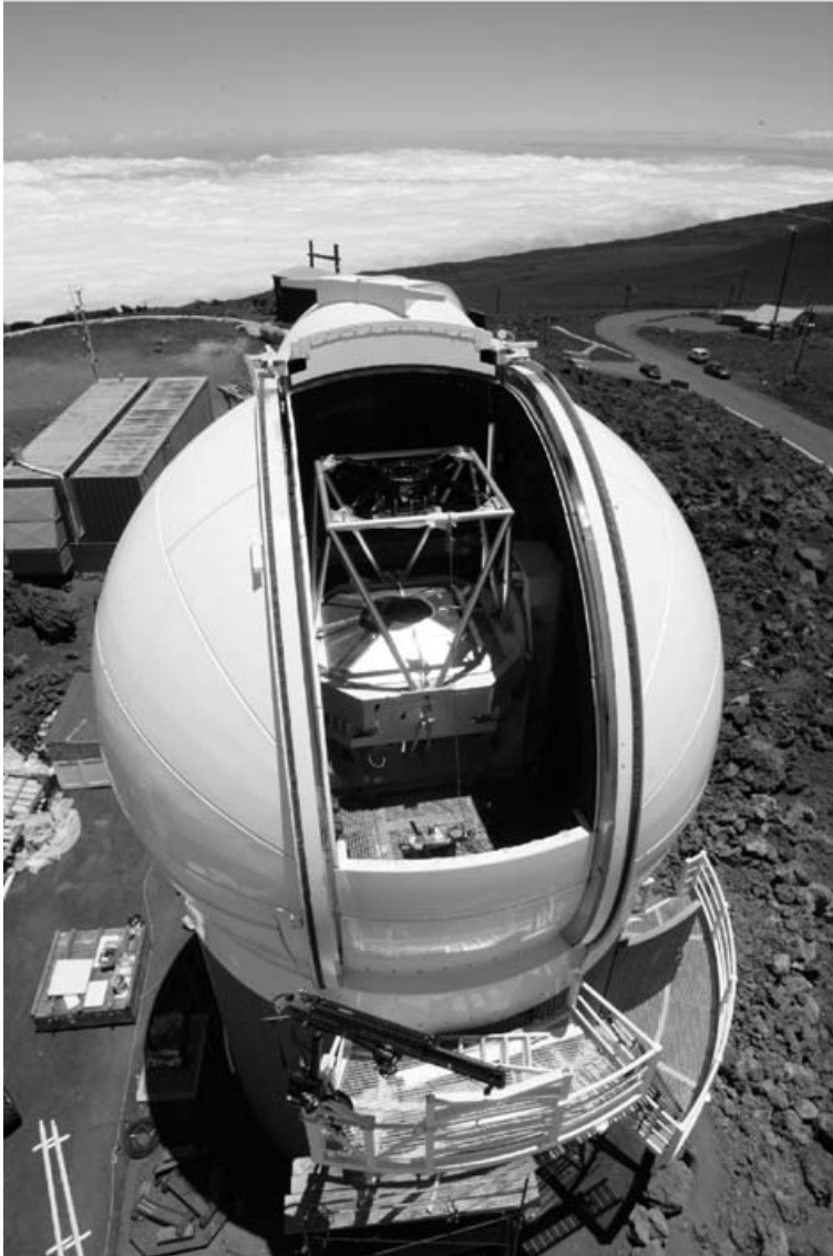
Figure 1. The prototype Pan-STARRS telescope installed near the top of Haleakala, Island of Maui, Hawaii. The main optics are in place, the dome is operational and first light has already occurred. Installation and testing of the OTA camera (in the hole at the center of the primary mirror) is the next step.
