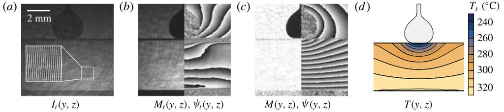
FIGURE 3. (Colour online) Leidenfrost interferometry experiment with an ethanol drop ( $R \sim \ell_c$ ,  $T_{imp} = 330^\circ\text{C}$ ), with interferogram  $I_t$  (a), magnitude  $M_t$  and (wrapped) phase  $\psi_t$  (b), background corrected magnitude  $M$  and phase  $\psi$  (c) and the reconstructed temperature field  $T(y, z)$  and drop contour (d). The wrapped phase is presented between  $-\pi$  (black) and  $\pi$  (white) for (b,c). All images are on the same scale.
