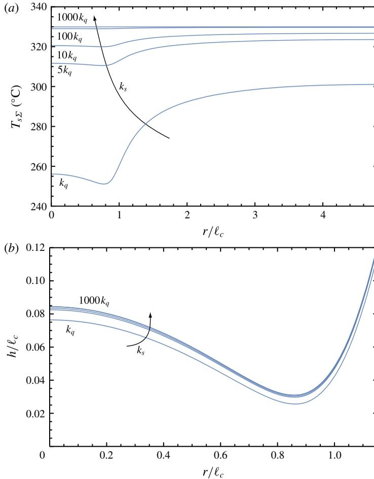
FIGURE 7. (Colour online) Effect of the variation of the substrate thermal conductivity  $k_s$  on the numerically predicted profiles of the substrate surface temperature (a) and the vapour film thickness (b) underneath a Leidenfrost ethanol drop of  $R = 1.37\ell_c$  with  $T_{imp} = 330^\circ\text{C}$  and the plate height ( $H_s = 4.5\text{ mm} \approx 3\ell_c$ ) as in the experiment. The value of  $k_s$  for the quartz used in the experiment is denoted by  $k_q$ .
