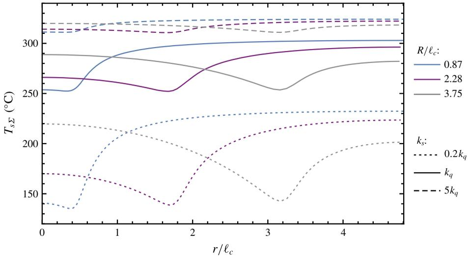
FIGURE 6. (Colour online) Numerically determined temperature profile at the top of the substrate underneath a Leidenfrost drop for different drop sizes and thermal conductivities of the substrate.  $H_s$  is taken at the value of the quartz plate height used in the experiment ( $H_s = H_q = 4.5$  mm).  $T_{imp} = 330^\circ\text{C}$  and  $k_q = 1.4 \text{ W m}^{-1} \text{ K}^{-1}$ , the thermal conductivity of quartz.
