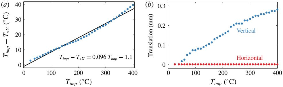
FIGURE 11. (Colour online) Temperature difference  $\Delta T = T_{imp} - T_{s\Sigma}$  across the quartz substrate in the absence of a drop (a) and the apparent translation relative to the reference interferogram (b).
