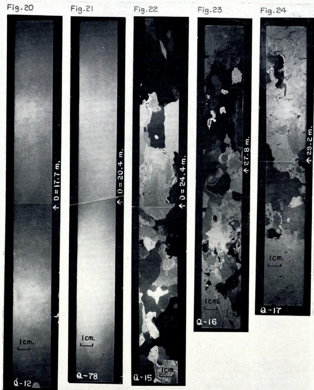
*Figs. 20-24. Vertical sections of basement ice photographed between crossed polaroids*
