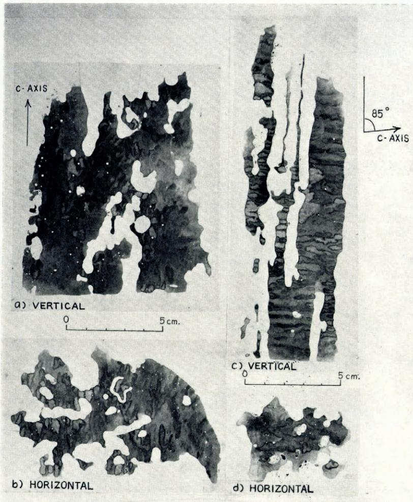
Fig. 2. Prints of cross-sections of candle ice. Sections (a) and (b) are of ice with  $c$ -axis vertical ( $\theta = 0^\circ$ ), while (c) and (d) are of ice with  $c$ -axis nearly horizontal ( $\theta = 85^\circ$ )
