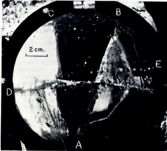
Fig. 12. Cross-section of ice of radial structure photographed between crossed polaroids
