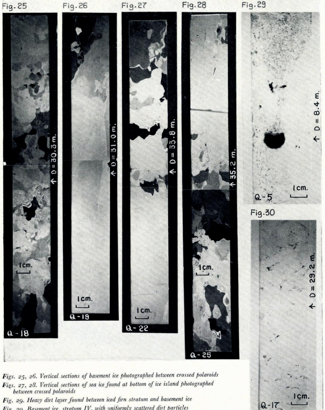
*Figs. 25, 26. Vertical sections of basement ice photographed between crossed polaroids*
