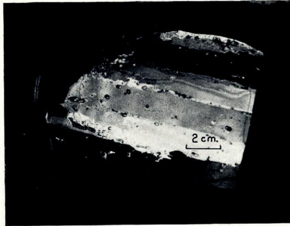
Fig. 1. Vertical cross-section of a bundle of candle ice between crossed polaroids
