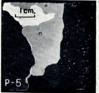
Fig. 45-51. Vertical and horizontal sections of sea ice samples from site P photographed between crossed polaroids
