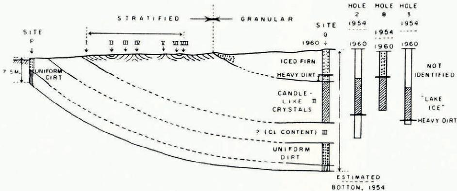
Fig. 52. A schematic diagram of the structure of T-3 (vertical exaggeration 6:1)
