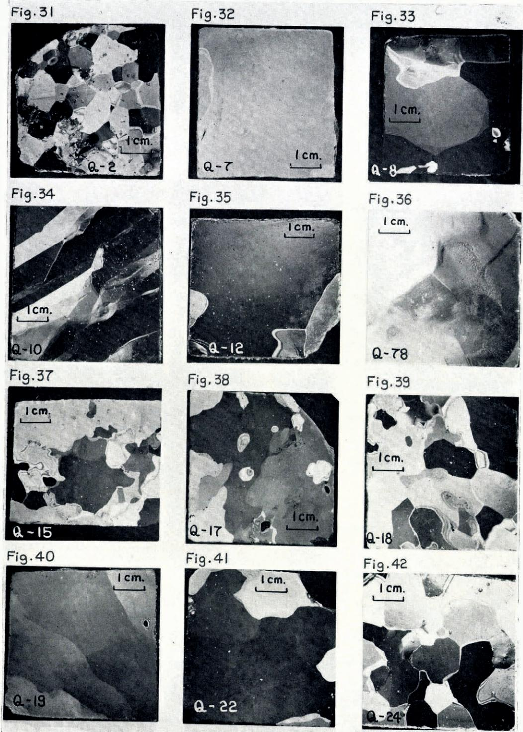
*Figs. 31-42. Horizontal sections of iced firn, basement ice, and sea ice photographed between crossed polaroids*
