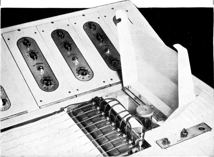
The new 8-channel E.E.G. is functionally designed to provide every possible facility. The long, low, desk-type instrument allows the seated operator a clear view of both patient and record, over three feet of the paper being visible at one time.
