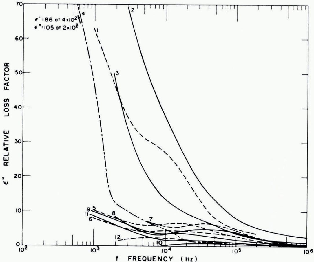
Fig. 15.  $\epsilon''$  as a function of frequency over the Debye dispersion range. Snow types given in the legend to Figure 14. (After Yosida and others, 1955; Watt and Maxwell, 1960.)
