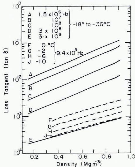
Fig. 23. Loss tangent as a function of density. (A-E, Yoshino, 1961; F-J, Cumming, 1952.)
