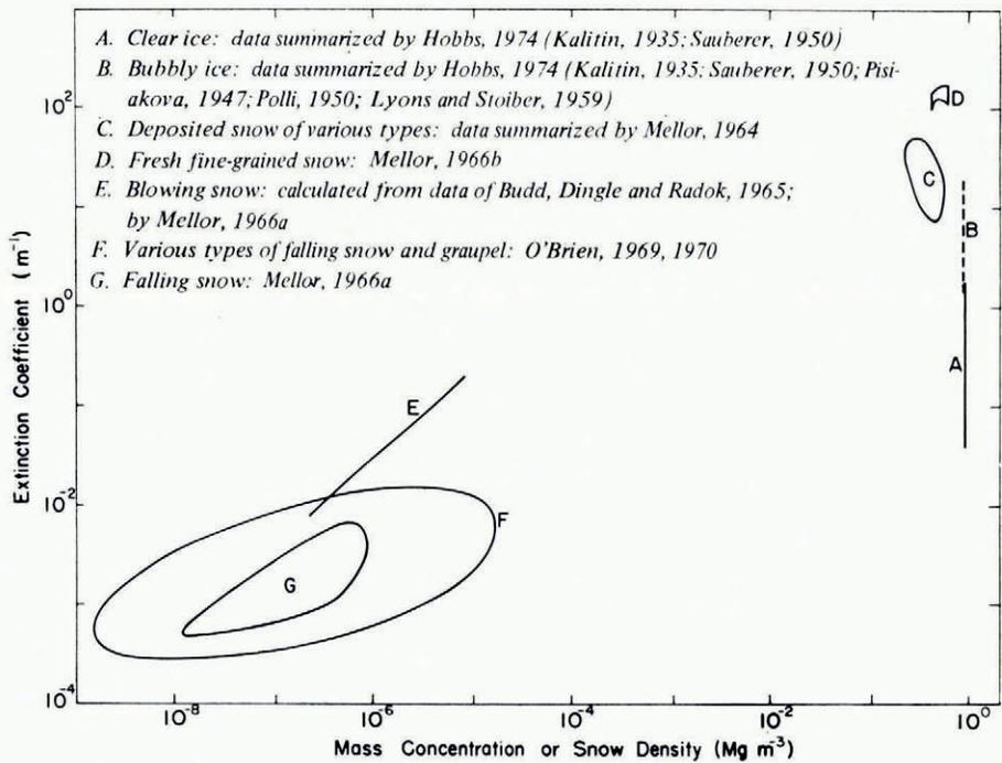
Fig. 29. Extinction coefficient plotted against density for a wide range of snow types. A 1 : 1 slope on this log-log plot would imply direct proportionality.
