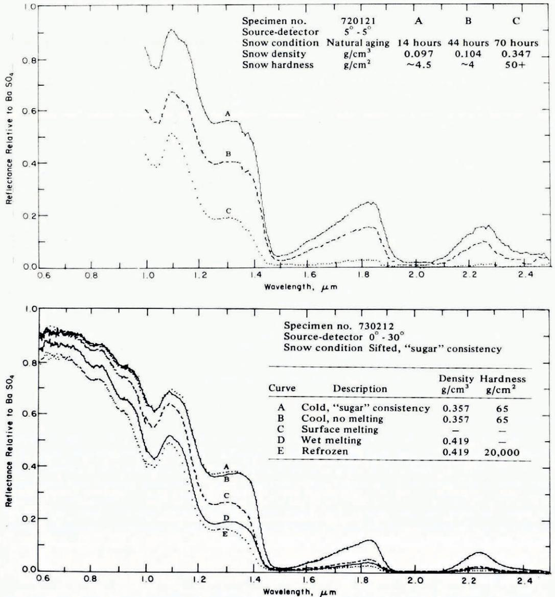
Fig. 38. Relative reflectance as a function of wavelength from the visible through the near infrared, showing effects of snow type and temperature. (From O'Brien and Munis, 1975.)
