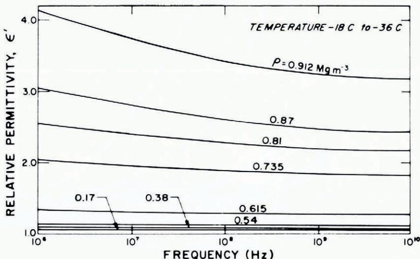
Fig. 16.  $\epsilon'$  as a function of frequency, from MF radio frequencies up to the radar K band. (After Yoshino, 1961.)
