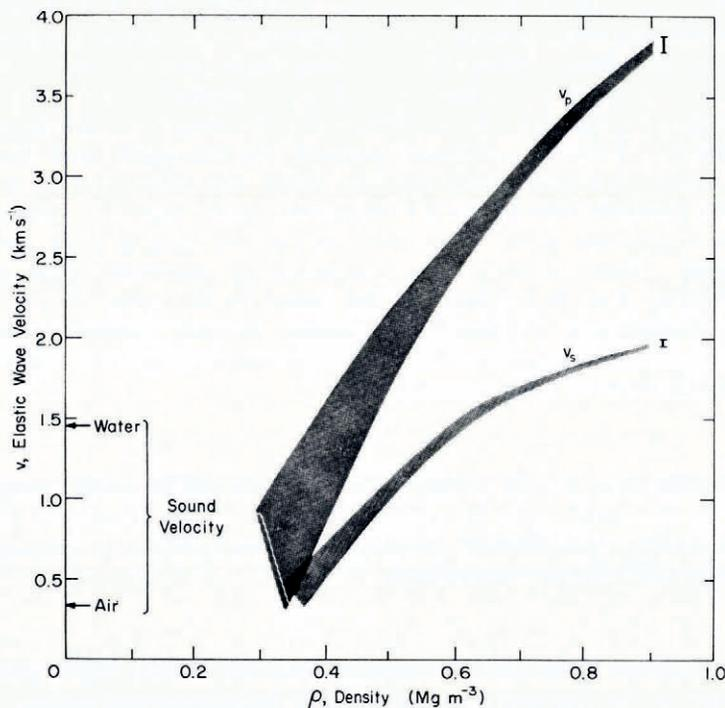
Fig. 5. Velocities of elastic waves as functions of snow density.
