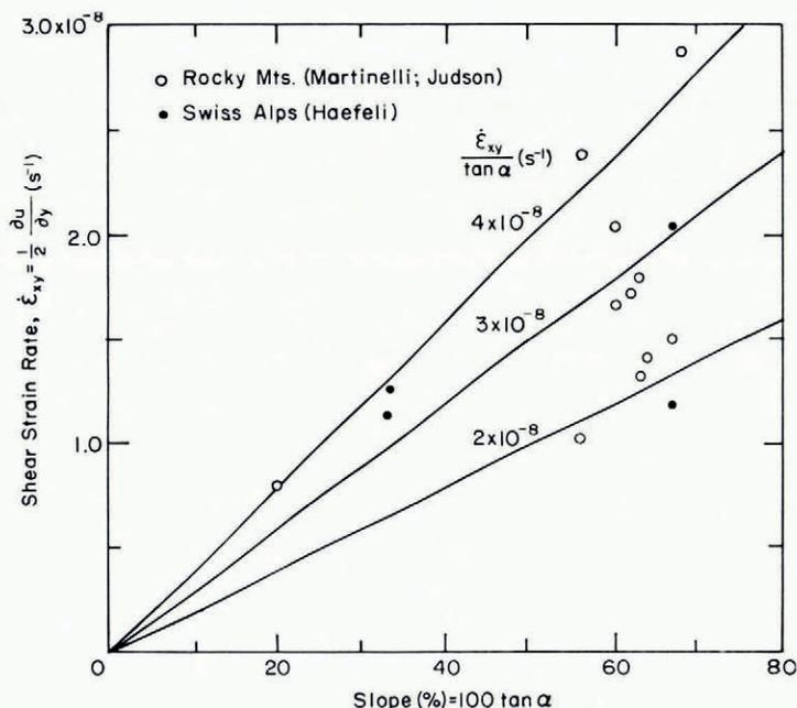
Fig. 10. Shear strain-rate as a function of slope for well-settled snow lying on a wide uniform slope. The arbitrarily drawn lines give different values of  $\dot{\epsilon}_{xy}/\tan \alpha$ .
