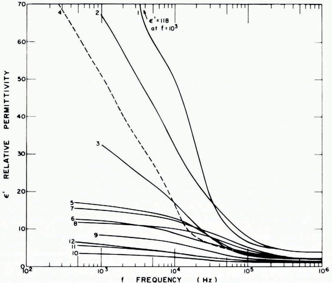
Fig. 14.  $\epsilon'$  as a function of frequency over the Debye dispersion range. (After Yosida and others, 1955; Watt and Maxwell, 1960.) Note: 1 and 4: Watt and Maxwell. 2, 3 and 5-12: Yosida and others.
