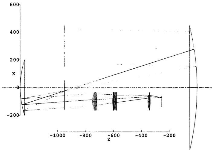
*Figure 2.* The optical scheme of the afocal telescope, with two parabolic mirrors and a dioptric objective.
