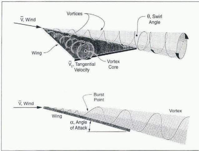
Fig. 3. Sketch of critical dimensions of vortex fence and vortex development.
