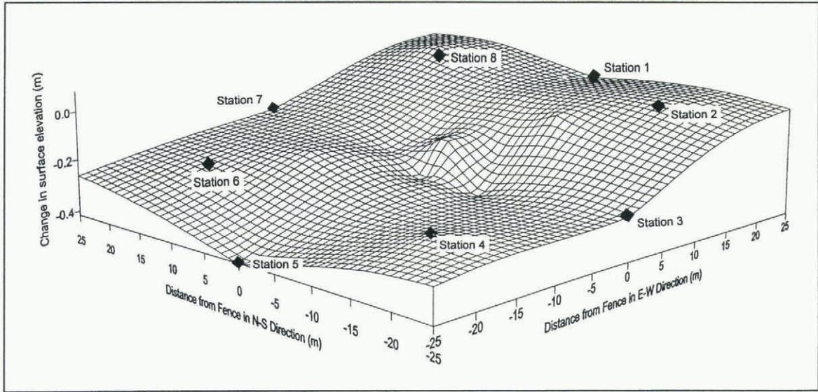
Fig. 7. Perspective map of snow-surface elevation change between 7 February and 28 June 1995, relative to the outboard survey point at station 1 (where no change in natural patterns was assumed). Outermost survey-target positions shown as solid diamonds.
