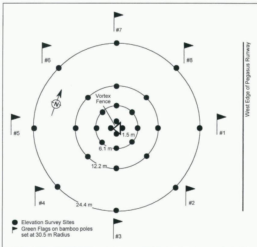
Fig. 5. Survey-target area for the full-scale vortex fence.
