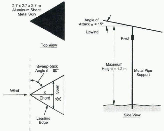
Fig. 2. Dimensions of the full-scale vortex fence.
