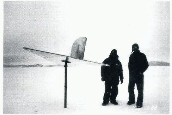
Fig. 4. Photograph of the installed vortex generator at Pegasus runway.
