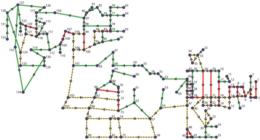
FIGURE 10. Linear stability of the trivial steady state for the large network example. The lines indicate the connections (pipes) and the circles indicate the junctions, which are numbered. The triangles indicate the direction of flow. The green dashed lines on black denote connections where the pathogens are predicted by the linear stability analysis to washout. The solid red lines indicate the connection where linear stability analysis predicts the pathogens persist and dotted yellow lines on black indicate the connections where the pathogens are predicted to be induced by upstream connections.
