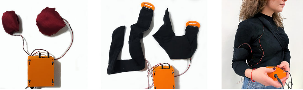
Figure 7. Two haptic modules, including Haptuator Mark 2 brand, type C and D actuators, are connected to the bluetooth audio amplifier. A 3D printed enclosure is designed for the amplifier and its power, audio input, and output connections. Elastic straps are designed to enclose the new haptic modules to fixture them on desired locations on the body. Fasteners are 3D printed to adjust the tightness and stability of the wearable straps.
