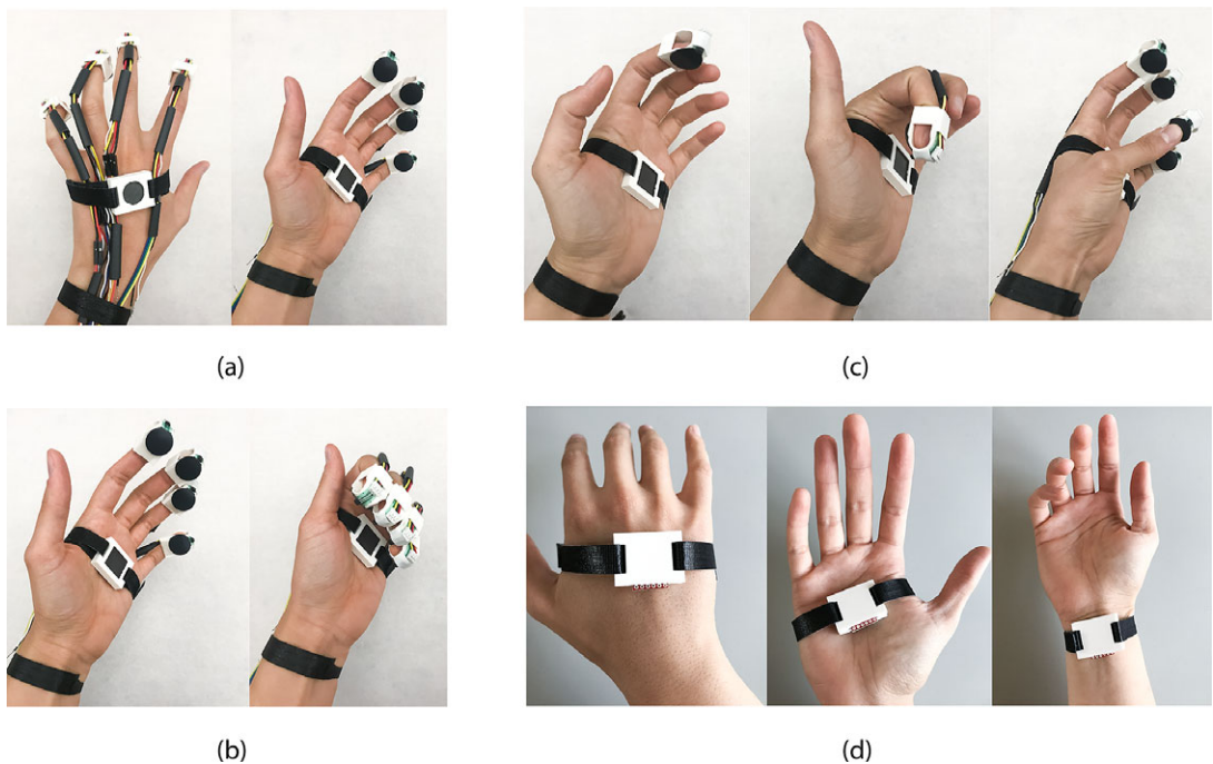
Figure 4. Felt Sound’s first prototype: (a) All modules are worn on one hand, (b) Fingertip sensor and a magnet module interaction change the state of the hall effect sensor while the FSR sensors output continuous data to control frequency, gain, and filter and effect parameters, (c) The hall effect sensors and the magnet placed on the palm allow detecting fist closing and opening gestures, and (d) Accelerometer module embedded into the 3D printed closure can be placed in multiple locations on the hand or wrist and coupled with other modules.
