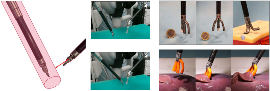
Figure 8. Left: a marker-less method tracks surgical tools, establishing VF geometry resembling to a cylinder with its central axis aligned with the instrument's axis [144]; right: the MUSH Hand II surgical tool, integrated on the dVRK robot [145–147].
