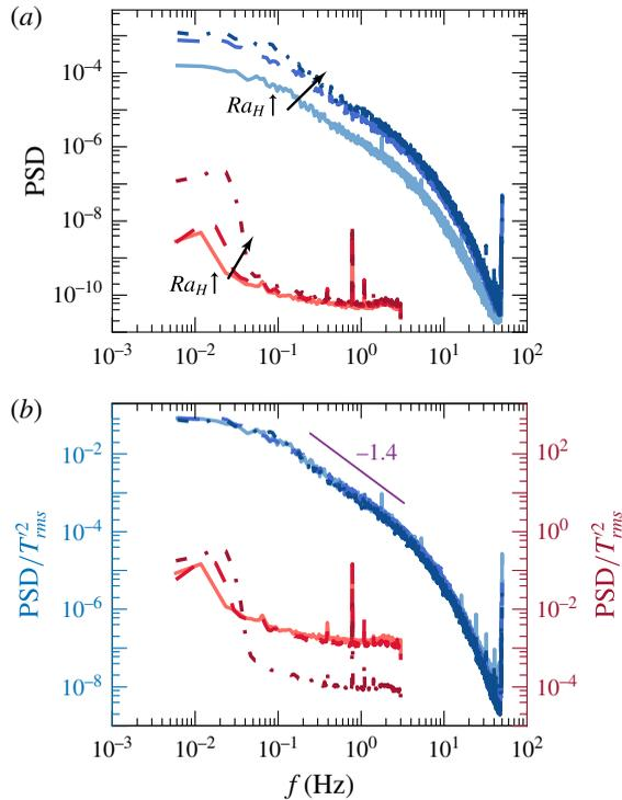
FIGURE 11. (Colour online) Raw (a) and normalised (b) power spectra of the temperature fluctuations at the centre of the set-up for single-phase (red lines) and two-phase  $\alpha = 0.9\%$  (blue lines): solid line,  $Ra_H = 5.2 \times 10^9$ ; dashed line,  $Ra_H = 1.6 \times 10^{10}$ ; dash-dotted line,  $Ra_H = 2.2 \times 10^{10}$ .
