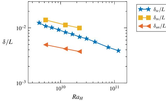
FIGURE 10. (Colour online) Normalised boundary layer thickness in the single-phase case as a function of  $Ra_H$ . Here  $\delta_{un}$  and  $\delta_{in}$  are numerically obtained thickness of the kinetic and thermal boundary layer, respectively. The thickness of the thermal boundary layer obtained from the experiments is given as  $\delta_{ie}$ .
