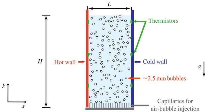
FIGURE 1. (Colour online) Rectangular bubbly column heated from one side wall and cooled from the other ( $H = 600$  mm,  $L = 230$  mm). Bubbles of approximately 2.5 mm diameter were injected through 180 capillaries placed at the bottom of the set-up (inner diameter 0.21 mm).
