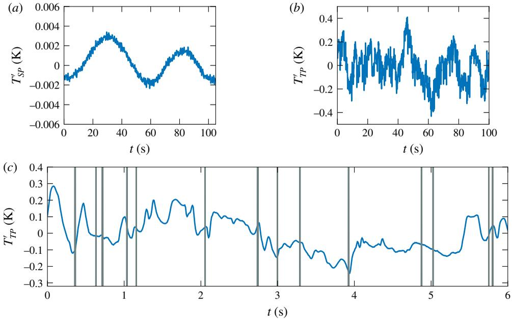
FIGURE 5. (Colour online) Signal of the temperature fluctuations at  $L = 11.5$  cm for  $Ra_H = 2.2 \times 10^{10}$  in (a) single-phase flow  $T'_{SP}$  (observed frequency of approximately  $10^{-2}$  Hz corresponds to large-scale circulation frequency, which is addressed in §4), (b) two-phase flow  $\alpha = 0.9\%$   $T'_{TP}$ , and (c) enlarged simultaneously obtained temperature fluctuations and optical fibre signal where each grey vertical line is a passage of a single bubble.
