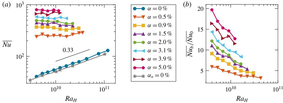
FIGURE 6. (Colour online) (a) Dependence of Nusselt number  $\overline{Nu}$  on the Rayleigh  $Ra_H$  number for different gas volume fractions ( $\alpha$ , experimental data;  $\alpha_n$ , numerical simulations); the size of the symbol corresponds to the error bar. (b) Heat transfer enhancement:  $\overline{Nu}_0$ , Nusselt number in single-phase case;  $\overline{Nu}_b$ , Nusselt number in bubbly flow.
