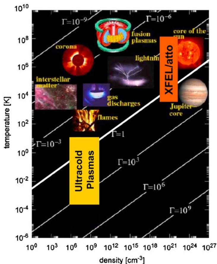
**Figure 1.** Natural and man-made plasmas in the density-temperature plane (after Ref. 1). Lines of equal Coulomb coupling parameter  $\Gamma$  (see text) are given in white, the thick white line corresponds to  $\Gamma = 1$ , the dividing line between ideal plasmas ( $\Gamma \ll 1$ ) and strongly coupled plasmas ( $\Gamma \gg 1$ ). Parameter ranges of the plasmas discussed here, are indicated by the yellow and orange bars for ultracold and laser pulse generated plasmas, respectively
