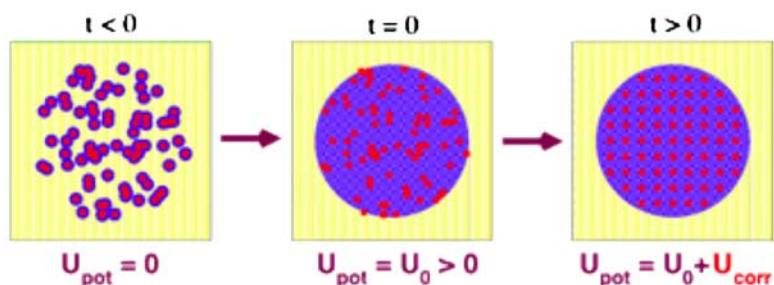
**Figure 3.** A gas with randomly placed atoms (left panel,  $t < 0$ ) is ionized at time  $t = 0$ . As a consequence, there is potential energy  $E_{\text{pot}} = U_0$  between the ions. Subsequently, correlations develop by which the potential energy is lowered, the generated positive correlation energy  $U_{\text{corr}}$  appears as kinetic energy (higher temperature) of the ions ( $t > 0$ )
