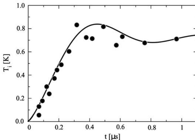
**Figure 8.** Calculated<sup>3</sup> (line) and measured<sup>13</sup> (points) ion temperature of an expanding plasma of 1 million strontium ions with initial density  $\rho = 2 \times 10^9/\text{cm}^3$  and initial electron temperature of  $T_e = 38 \text{ K}$
