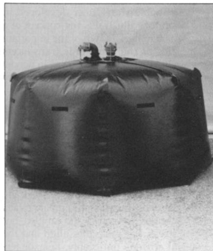
▲ **Collapsible Storage Tank with Replaceable Liner:** The ZipTank from ILC Dover provides temporary storage in a two-component system featuring a high-strength fabric outer restraint and a chemically resistant, replaceable inner liner. The ZipTank folds for storage when not in use, and the replaceable liner permits sequential storage of incompatible products. Fugitive emissions and air contaminations are eliminated because the tank collapses to fluid level.
