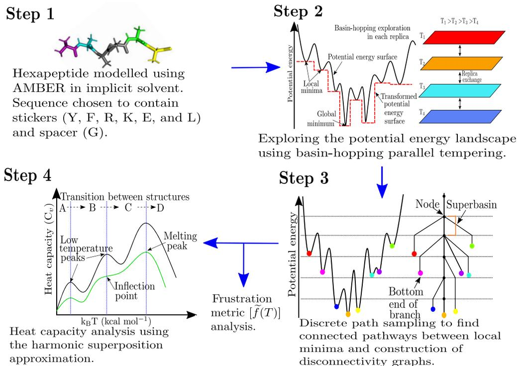
**Figure 1.** Schematic figure representing the workflow for the computational potential energy landscape exploration to interrogate peptides of varying phase separation propensities.
