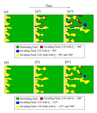
Figure 21. Comparison of invasion morphologies obtained using the 2-D model for two distinct effective contact angles, namely (a-a'')  $\theta_e=90^\circ$ , and (b-b'')  $\theta_e=135^\circ$ , with that obtained for  $\theta=180^\circ$  (baseline) used to carry out the 2-D numerical simulations presented above. The three columns depict the invasion patterns recorded at three different time steps. The capillary number is intermediate:  $\log(Ca)=-4.0$ .
