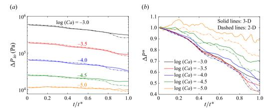
Figure 14. (a) Average pressure drop  $\Delta P_{io}$  between the inlet and outlet of the fracture, as a function of time (normalised by the breakthrough time), for different Ca values. (b) Normalised average pressure drop,  $\Delta P^* (= \Delta P_{io}/\Delta P_{io}(t=0))$  as a function of time. The solid and dashed lines correspond to the 3-D and 2-D simulation results, respectively.
