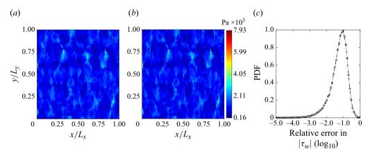
Figure 25. Wall shear stress distribution  $|\tau_w|$ , in Pa unit, resulting from the top and bottom wall surfaces of the fracture, for the 2-D (a) and 3-D (b) models at Re = 10.0. (c) The PDFs of the logarithm of the relative errors between (a) and (b) are shown in (c). The dot-dashed line is simply a broken line linking the symbols.
