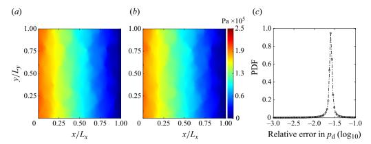
Figure 24. (a,b) Dynamic fluid pressure  $(p_d)$  distribution for the 2-D (a) and 3-D models (b), for Re = 10.0. (c) The PDFs of the logarithm of the relative errors between (a) and (b). The dot-dashed line is simply a broken line linking the symbols.
