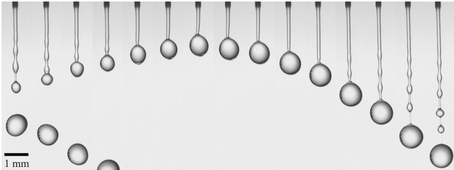
FIGURE 1. The ‘gobbling’ phenomenon: a large terminal drop periodically develops at the end of a thin jet of a viscoelastic fluid (100 p.p.m. of polyacrylamide in aqueous solution). The drop initially moves upward, ‘gobbling’ the thread, before detaching. The time interval between the images is 6 ms (figure from Clasen et al. 2009).
