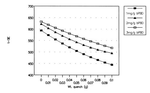
Fig 1. Plot of t-SIE vs weight of quenching agent added (5% acetone in benzene), bis - MSB fixed at 3 mg.g<sup>-1</sup> benzene, butyl - PBD = 1, 2 or  $3mg.g^{-1}$
