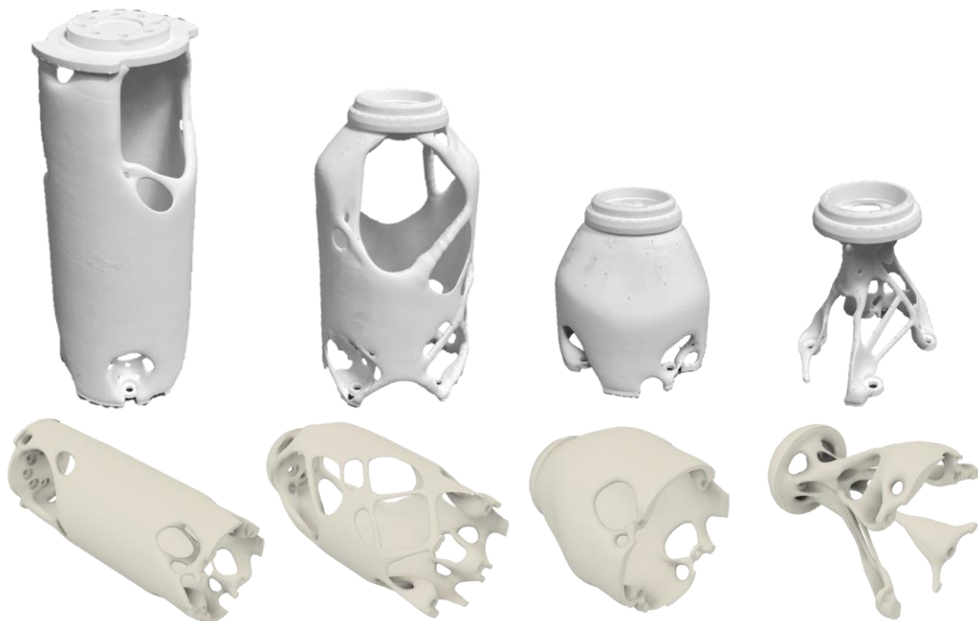
Figure 4. Optimised parts from OSE1 (left) to OSE4 (right). The top row shows the 3D printed parts and the bottom row shows the CAD representation
