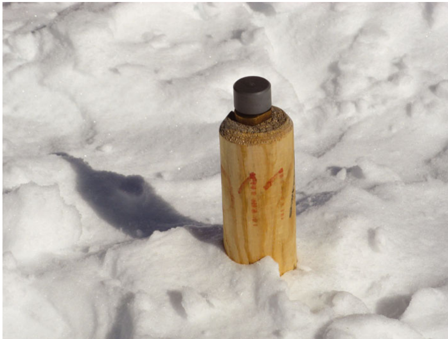
Fig. 2. Example of a GNSS marker in the southern part of Vostok Subglacial Lake (marker 9). The wooden stake extends to a depth of \sim 60 cm into the firn. On top of the stake a special screw is fixed onto which the GNSS antenna is mounted. After the occupation, a plastic cap (grey) is used to protect the screw thread.
