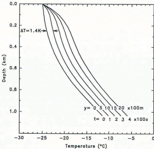
Fig. 7. Temperature in the margin as a function of distance  $y$  from the outer edge for a constant transverse velocity  $v$  of  $5 \text{ m a}^{-1}$ . The corresponding residence time  $t$  of the ice in the margin is also shown.
