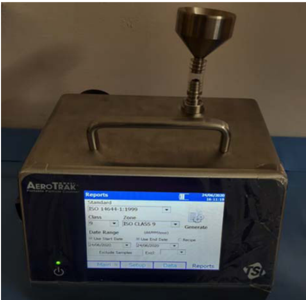
Fig. 2. Portable particle counter placed at a far distance from the site of drilling inside the operating theatre.
