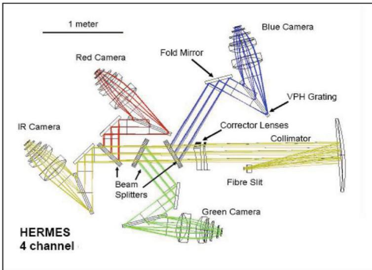
**Figure 1.** Optical design of the HERMES four-band high-resolution spectrograph.
