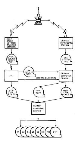
Figure 3 - Helios System Data Flow
