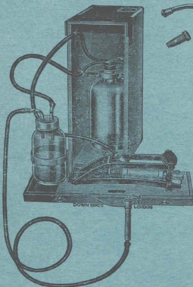
Specially designed trigger operated suction tube handle, which prevents loss of vacuum in the circuit
