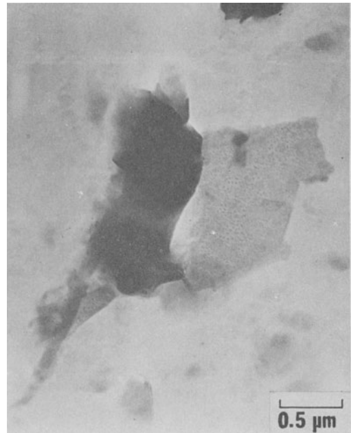
Fig. 5. Typical thin and subhedral mica, and a rather thick and irregular montmorillonite aggregate in the Cheto sample.
