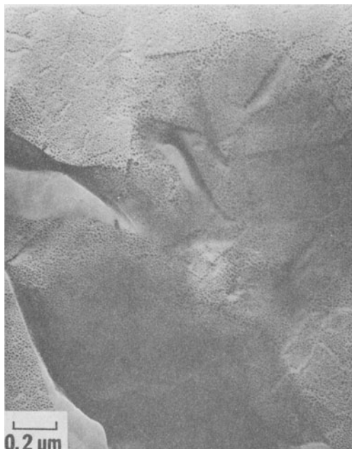
Fig. 9. The transmission electron image of a thin, flat aggregate of crystallites in the Wyoming montmorillonite.
