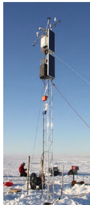
Figure 1. Listing of major components of the AMIGOS station (left) and sketch of an idealized installation of the AMIGOS-3 ice-ocean-atmosphere station (center). Installed AMIGOS-3a at Cavity Camp, TEIS in January 2020 (right). See also Appendix, Table S1 and Figures S1a, S1b and S2.
