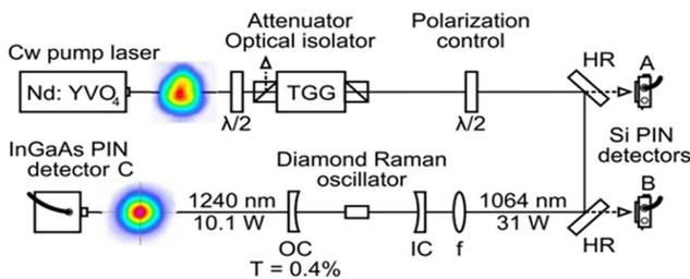
Figure 4. Schema of the external cavity DRL<sup>[31]</sup>.
