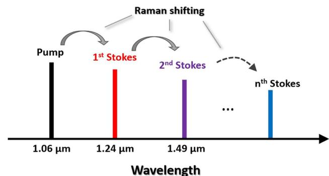
**Figure 8.** Schematic of a cascaded DRL pumped by a 1.06  $\mu\text{m}$  laser<sup>[20]</sup>.
