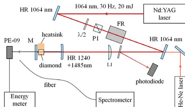
**Figure 3.** Schematic of the external cavity Raman laser<sup>[67]</sup>.
