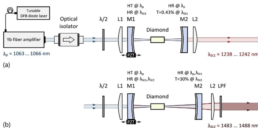
**Figure 6.** Experimental setup of the tunable (a) first-order and (b) second-order Stokes DRL operating in SLM<sup>[70]</sup>.
