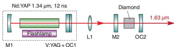
**Figure 2.** Schematic of the laser system consisting of a pumping Nd:YAP laser and DRL<sup>[66]</sup>.
