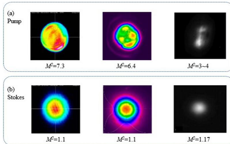
**Figure 7.** Spot distribution of pump and Stokes beams in DRLs<sup>[37,83,84]</sup>: (a) pump spot distribution; (b) corresponding Stokes spot distribution.
