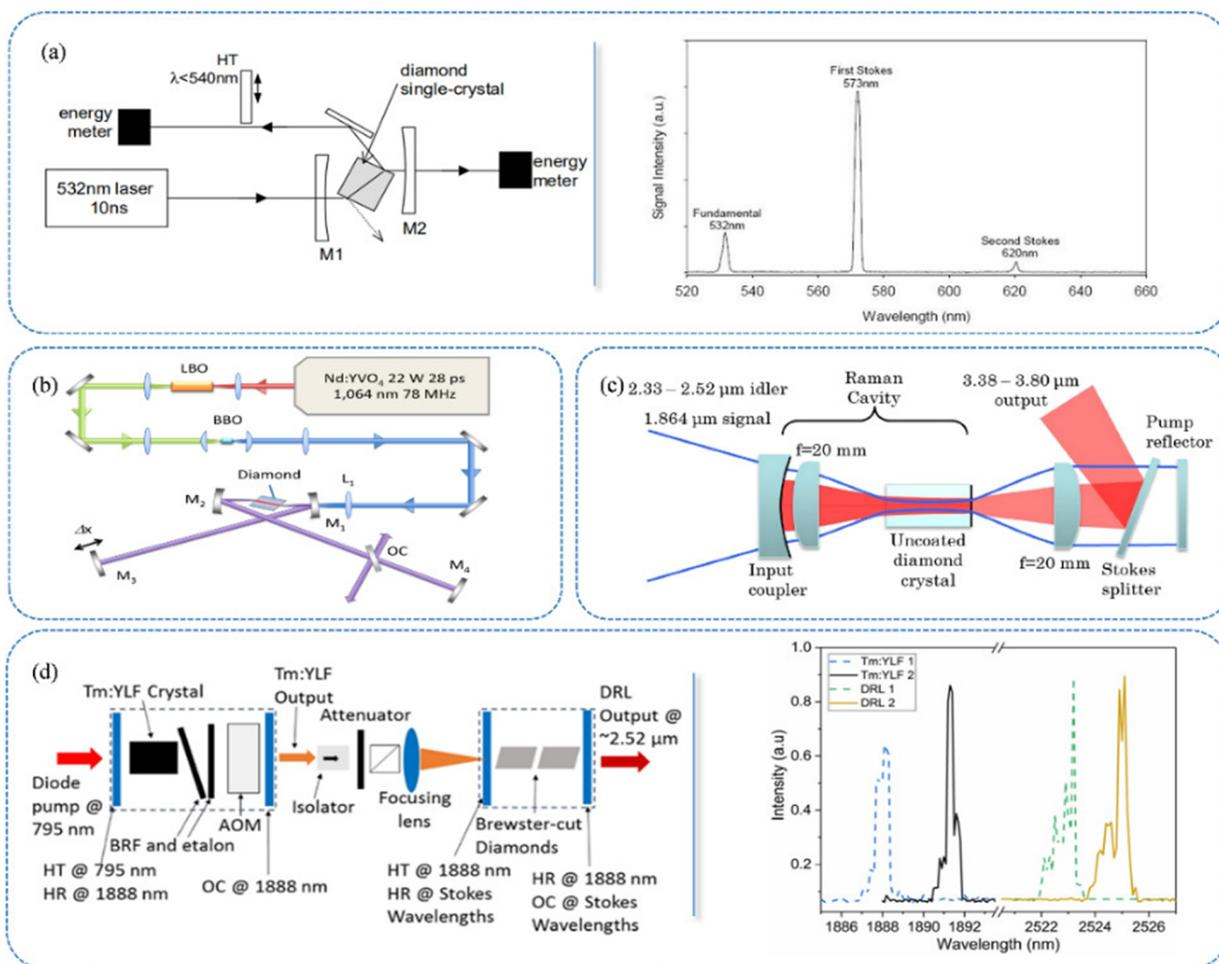
**Figure 9.** Different wave bands of DRLs and the related output spectra<sup>[7,90–92]</sup>: (a) 573 nm and 620 nm laser output from 532 nm pump beam; (b) 275.7 nm laser output from 266 nm pump beam; (c) 3.38–3.8  $\mu$ m laser output from 2.33–2.52  $\mu$ m pump beam; (d) ~2.53  $\mu$ m laser output from 1.89  $\mu$ m pump beam.
