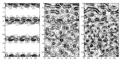
**Figure 2.** Contours of  $u_x$  (top),  $\Theta$  (middle) and  $u_z$  (bottom) are shown in a horizontal xy-plane.  $R = 5 \times 10^4$  (left),  $R = 2.5 \times 10^5$  (middle),  $R = 1 \times 10^6$  (right),  $\tau = 10^3$ ,  $P_r = 7.0$ , non-slip side walls.
