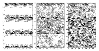
Figure 1. Contours of  $u_x$  (top),  $\Theta$ (middle) and  $u_z$  (bottom) are shown in a horizontal xy-plane.  $R = 7 \times 10^4$  (left),  $R = 2.5 \times 10^5$  (middle),  $R = 2.5 \times 10^6$  (right),  $\tau = 10^3$ ,  $\Gamma = 2$ ,  $P_r = 7.0$ , stress-free b.c.
